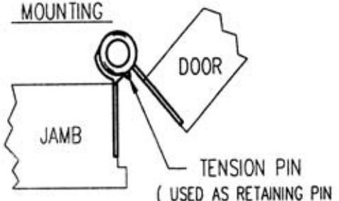
THIS HINGE CAN BE USED FOR RIGHT HAND, LEFT HAND, AND PAIRS OF DOORS WITHOUT CHANGING THE APPEARANCE. TO OBTAIN OPPOSITE HAND, TURN HINGE UPSIDE DOWN.
