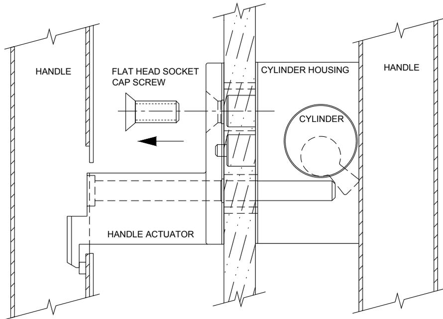
3. Pull handle away from glass. Remove handle actuator from handle.
