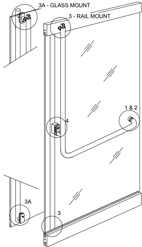
1. Push exterior horizontal handle retainer with rubber bushing through glass hole from interior side, into horizontal handle, and tighten with spanner wrench.
