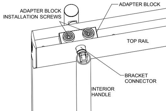
Install the Adapter Block into the Bottom Rail. Insert the handle fitting into the Adapter Block and tighten the setscrew.
