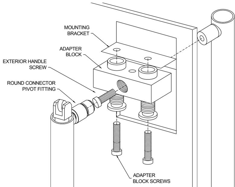
At the bottom Adapter Block, loosen up socket set screw and pull exterior handle away loose.
