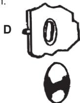
**D.** Concealed latch and emergency cover plate. Latch has a fully concealed case made of Zamac No. 3 castings with stainless steel bolt and mortised face plates fully tamper and theft proof. Cover plate is a Zamac No. 3 chrome plated casting which snaps in place. This has a slot for emergency entrance feature as standard.
