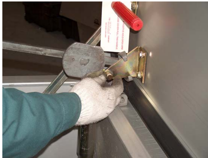
Figure 3b TL-03 (for small steel springs)
