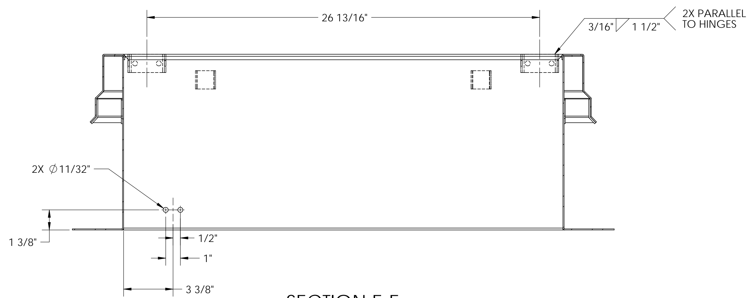
SECTION E-E HINGE SIDE
