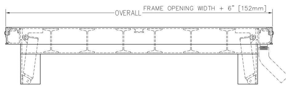
Frame areas that come in contact with concrete shall be coated with bituminous paint
