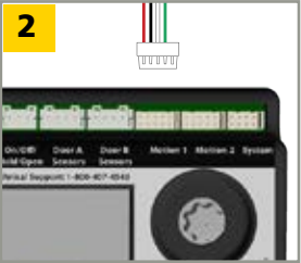
Plug Eagle Harness(es) into hub port labeled Motion 1 and, if applicable, Motion 2 .
