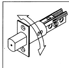
b. Insert deadbolt. Install with two #8 x 3/4" flat head combination screws provided (see diagram for proper positioning). Ensure deadbolt head is extended throughout installation procedure.
