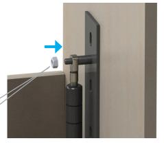
Screw nuts on top and bottom to secure pistons.
