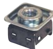
Item #: GD3066 - Leg Bushing Insert bushing for 1" Square Legs, threaded 1/4" - 20, use with Glides. Insert to bottom of Square Leg (RV28S).
