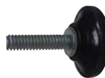
Item #: GI643-411-081 Black Threaded Glide 1-1/8" Diameter, 1/4-20 threaded stem, length 1", Non-swivel, standard duty, polyethylene plastic guide. Insert Glide into Leg Bushing (GD3066).
