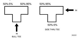
• On a side/thru tee, the side outlet must always be the smallest of the two splits.
