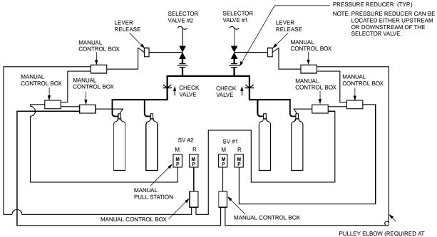
PULLEY ELBOW (REQUIRED AT EACH CHANGE IN DIRECTION)
