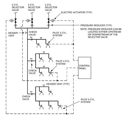
EXAMPLE NO. 2 (TYPICAL SELECTOR VALVE INSTALLATION - ELECTRIC ACTUATION)
