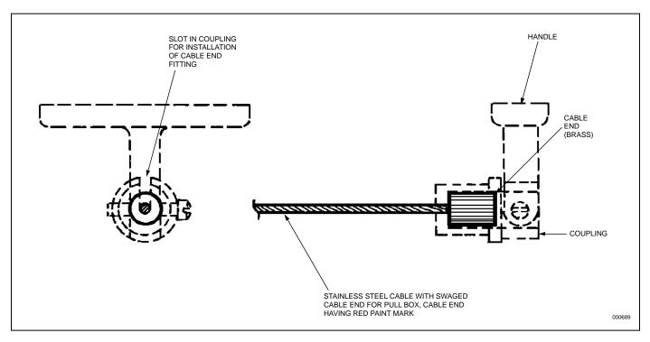
NOTE: The strength of the end fitting exceeds the breaking point of the cable.
