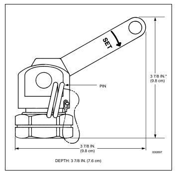
\* Add 1 9/16 in. (3.9 cm) to height when lever is in the straight up position.
