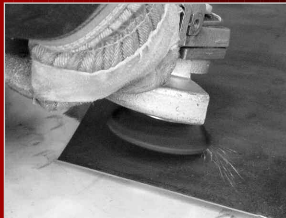
The aggressive impact action of Anderson's knot cup brushes make them suitable for a wide range of heavy-duty cleaning applications.
