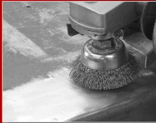
Removing paint from large surfaces is accomplished easily with an Anderson crimped wire cup brush mounted onto your right angle grinder.
