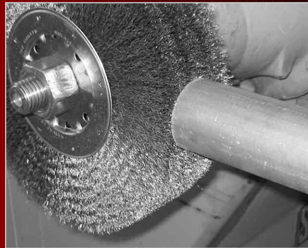
Whether they are gang-mounted or used individually, crimped wire wheels offer an effective, economical solution to deburring the ends of tubes after cutting.
