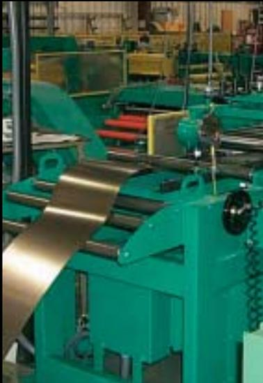
Amweld's roll-forming technology produces frames with the tightest tolerances in the industry.
