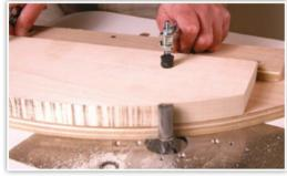
When shaping curved stock with a template, extend template beyond the work-piece so that the template contacts the guide bearing before work-piece contacts the bit.
