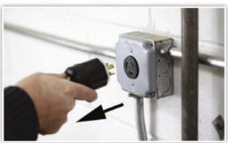
3. Disconnect the power tool from the power source before changing the saw blade.
