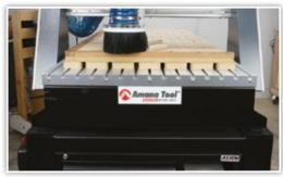
**25.** Dust collection system and vacuum systems will aid in a fires speed travel. A tool left running in the same place for a sufficient amount of time, can and will start a fire. It is essential to never leave a CNC running without an operator.
