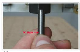
26. Proper Tool Installation – To ensure proper fit and prevent unnecessary strain on the collet, use the collet designed to fit your shank diameter. The tool's flute should never extend into the collet and should always be inserted up to the straight line on the 'K' mark on all of the Amana Tools bits.
