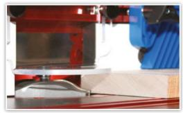
18. Always plan to route in several passes to achieve the final profile. Do not force the bit into the work-piece. If the router is straining or becomes overloaded, the cut is too heavy or bit is dull.
