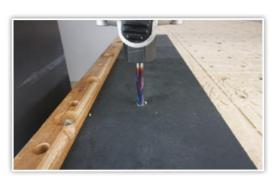
**27.** Never start the machine with the tool in contact with the work piece.
