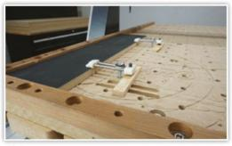
Always secure your work piece to the spoilboard using clamps, vacuum or double-sided tape. Never try to hold any work piece on the table by hand.
