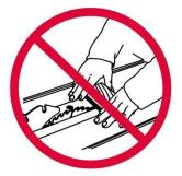
**4.** Never cut stock freehand. Always use the fence or miter gauge to support the work-piece.
