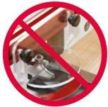
Never start the router with the router bit in contact with the stock/work-piece.
