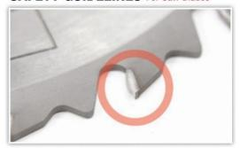
Do not use a blade that is cracked or broken, has a chipped or missing tooth, or has been dropped or damaged.
