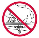
5. Never use a large diameter bit in a handheld router. Refer to Amana Tool® website and catalog for guidelines.
