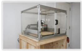
For smaller size CNC machines we recommend the use of an enclosure, this will not only help contain dust and noise, but will add an extra layer of safety in the event anything flying off of the machine.
