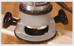
6. Plan the cutting path to avoid cutting the power cord.
