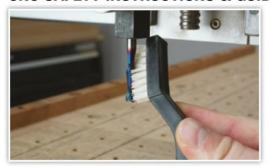
**15.** Keep bits clean and sharp for best results and performance. Do not use dull or damaged tools.
