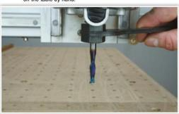
19. Make sure the collet is securely tightened after installing your cutting tool. Any unsecured cutting tool may fly loose from the collet and cause serious injury and damage.
