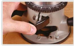
8. Secure the router motor in the base before plugging it in to the power outlet.
