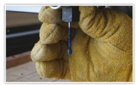
Never touch a cutting tool immediately after use, as it may be hot. Use caution when handling the collet and spindle nut. Keep an oven mitt or heavy glove handy.
