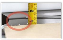
Before starting the saw, adjust the saw blade height 1/8" above the work-piece.
