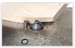
${\bf 21.}\ \ {\bf Use}$  a starting pin when shaping curved stock without the use of a template.
