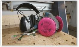
**3.** Always wear hearing protection, safety glasses or face shield, dust mask and safety clothing even during short periods of operation
