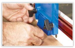
Always use featherboards to hold the work-piece firmly to the table and fence.
