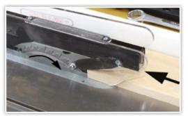
Always feed the stock against the direction of the power tool rotation.
