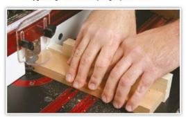
19. Use a jig or miter gauge when shaping end of narrow stock.
