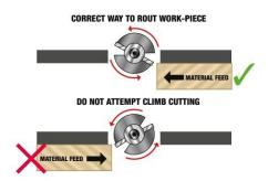
**16.** Never "climb" cut. Always feed the work-piece against the rotation of the bit.
