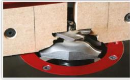
**20.** Reduce the fence opening as much as possible in order to provide support for the work-piece. When using large diameter bits, such as a raised panel bit, make a zero-clearance fence opening.
