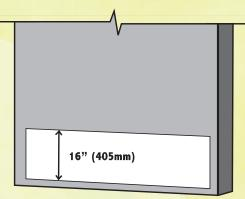
Unless otherwise tested and approved, protection plates are to be located within the lower 16" (405mm) area of the door.
