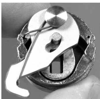
Fig. 2h: Ready for LH operation.
