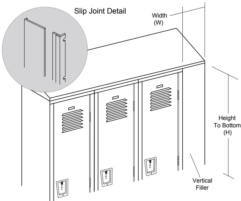
20 ga. commercial grade steel, powder coated to match locker color. Filler formed into an angle and connected with slip joints to create a smooth finish.
