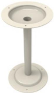
Pedestal fabricated of 1-1/2" diameter steel tubing with 10 ga. steel flanges welded to each end. 16-1/4" high; powder coated to match lockers, or available in our standard black and almond colors.
