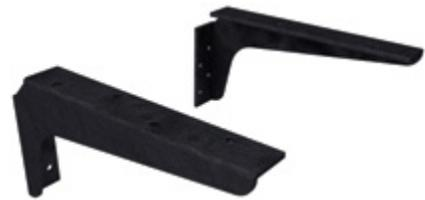
1 1/2" wide reversible steel bracket. Span between brackets not recommended to exceed four feet. Available in black, almond, or stainless steel.
