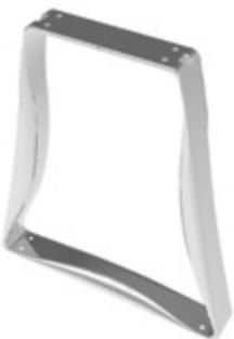
Stainless Steel, #4 Satin Finish, 2" wide, 16 ga. brushed stainless steel, 16 1/4" high formed to trapezoidal shape. Pedestal has four mounting holes in the top for fastening to the bench, and four holes on the bottom, for mounting into the floor.
