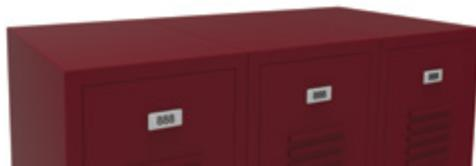
18 ga. commercial grade steel, powder coated to match locker color. Continuous slope tops up to 72" in length (longer lengths connected with splices). Degree of slope is 1/3 of locker depth.
