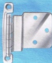
NO. 552 SEMI-CONCEALED HINGE \frac{3}{8} " Inset Only Length of barrel 1\frac{1}{2} " Length of Pad 2"
