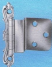
995 SEMI-CONCEALED HINGE 3/8" Inset • 1 1/2" Barrel Length 2" Pad Length.
