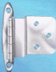
NO. 555 DELUXE SEMI-CONCEALED HINGE \frac{3}{8} " Inset Only. Length of barrel 1\frac{1}{2} " Length of Pad 2" Pat. No. D-182,889 Canadian Pat. No. RD1957
