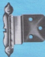
865 SEMI-CONCEALED HINGE 3/8" Inset 1 1/2" Barrel Length 2" Pad Length Pat. No. D-215,816
