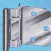
NO. 580 SEMI-CONCEALED "WRAP AROUND" HINGE FOR \frac{3}{8} " INSET DOORS Size: 1\frac{3}{4} " x 1\frac{3}{4} " Length of Barrel 1\frac{1}{4} " Length of Pad \frac{7}{8} "
