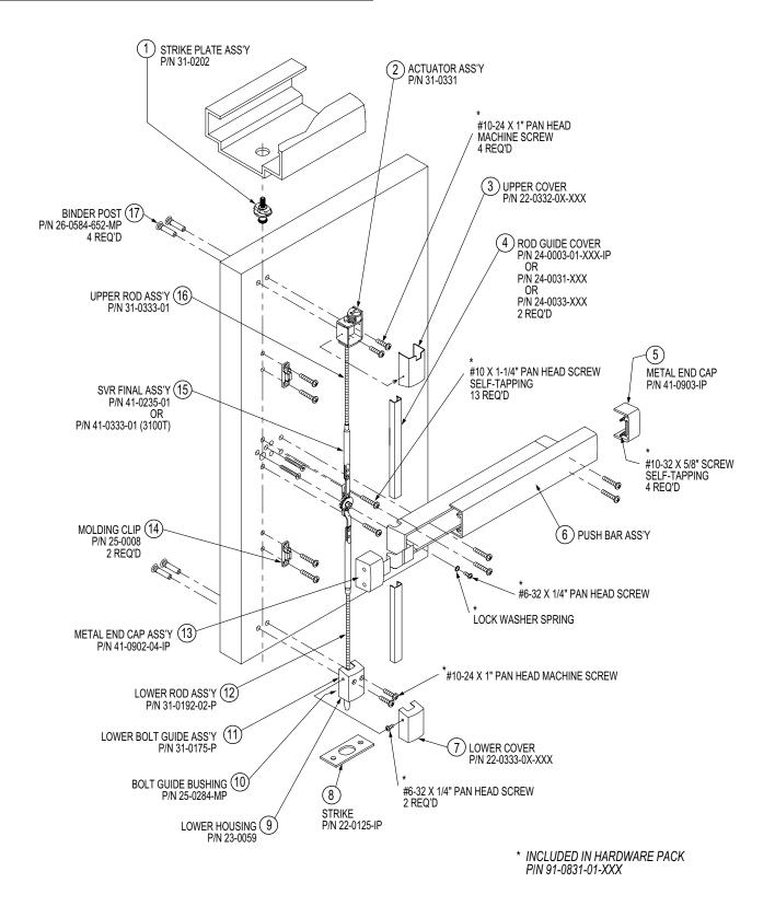
3100 Series Surface Vertical Rod Exit Device (Including 3100T)
