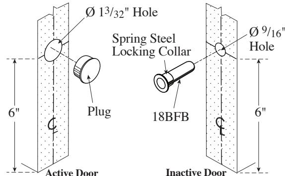
NOTE: Thermal pin to be centered in door thickness;
