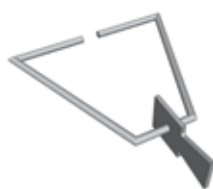
#107 Dovetail Horizontal Triangular Tie: 1/8" clip with 3/16" dia. wire tie.
