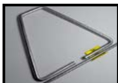
#370 welded to #316 Triangle
