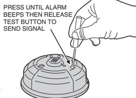
PRESS UNTIL ALARM BEEPS THEN RELEASE TEST BUTTON TO SEND SIGNAL
