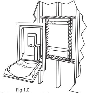
3. The unit comes with two mounting brackets that need to be secured to the mounting frame as shown in Fig 1.0.
