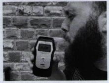
**STEP 4**. Get the test subject to breathe normally and then blow in a continuous stream into the tube. The unit will emit a continuous beep during the blow and then stop when the sample is complete.
