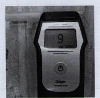
STEP 5. After the sample the unit will read <ANALYSING> and then give a number, which is a measurement of the alcohol per ml of blood. The MAXIMUM permissible is 35microgrammes of alcohol per 100ml of breath. So the reading needs to be below 35
