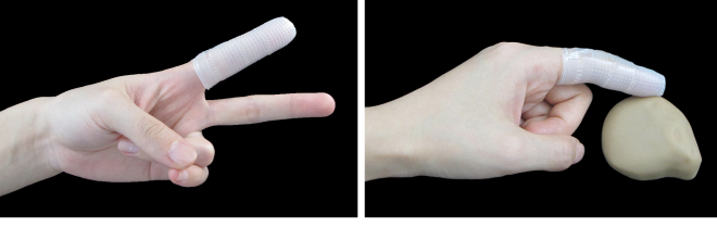
Fig. 1: Wearable sensing prototypes based on a similar device design to that employed in this paper. Such sensors may prove useful for wearable sensing during physical examinations by palpation.
