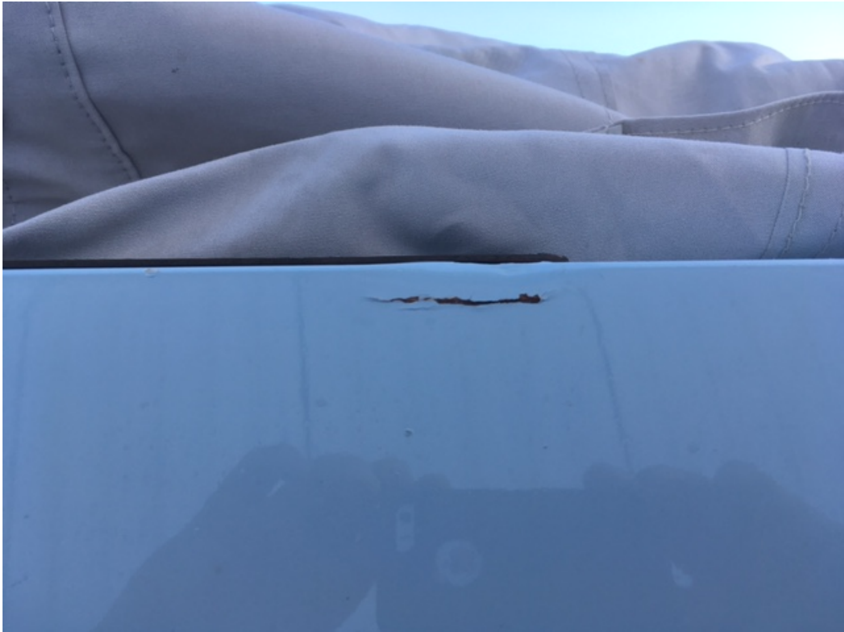
Sprig damage from Scoundrel at forward end of Jib tracks
