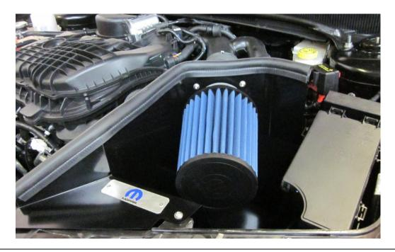
h) Attach the Mopar air filter to the air intake tube. Check all clearances and tighten all nuts, bolts and hose clamps installed in previous steps.
