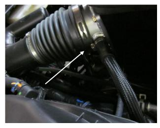
g) Attach the breather hose to the air Intake tube and secure it with the supplied #12 hose clamp
