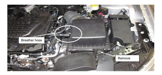
e) Remove the valve cover breather hose from the air box and remove the M8 bolt from the air box stay.
