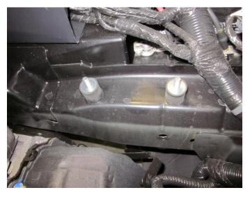
c) Install the 2 included rubber mounted studs in place of the factory studs.
