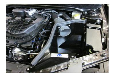
f) Attach Mopar air intake tube to the factory rubber hose and secure the heat shield to the rubber mounted studs with the M8 nuts. Mount the heat shield air guide to the radiator support with the M6 hardware.
