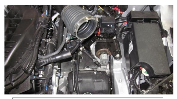
h) Once the previous steps have been completed, detach the air box from the factory intake tube. The air box can then be lifted up and out of the engine bay.
