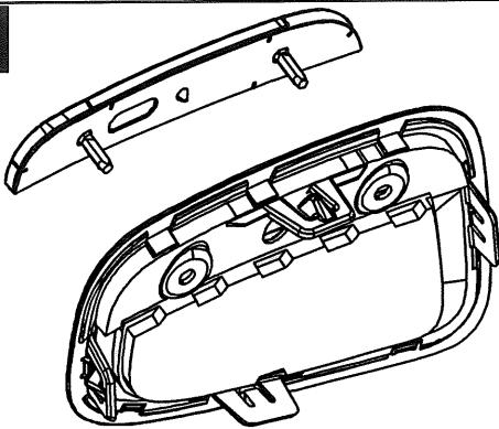
Remove fasteners from rear side bezel to remove reflector. Install reflector on supplied rear side bezel (Item E). Repeat for opposite side
