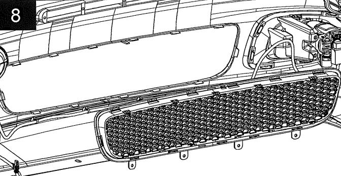
Remove lower grille from opening. A pry tool may be required for this step. Install supplied lowered grille (Item A) to fascia. Ensure all clips are fully engaged by applying pressure at each clip location.
