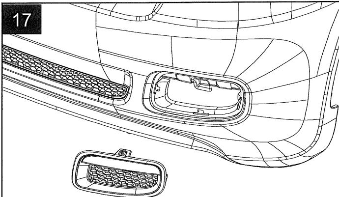
Remove rear side reflector bezel. A pry tool may be needed in this step. Repeat for opposite side.
