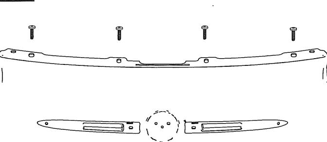
Remove bolts at top of fascia using a T30 Torx bit. Completely remove front fascia from vehicle. Save bolts for re-installation.
