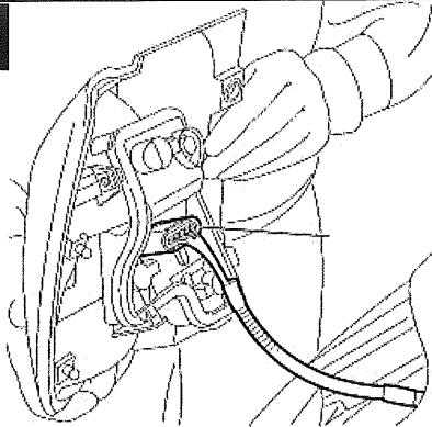
Disconnect rear tail lamp wire harness. Set Tail lamp aside for re-installation.
