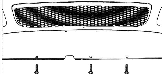
Remove 3 bolts from underside of front Fascia using T30 Torx bit. Save bolts for re-installation.
