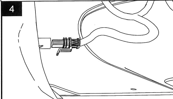
Disconnect fog light wire harness at drivers side of radiator support.
