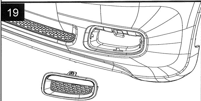
Install supplied Rear Side Reflector bezel (Item E). Ensure all clips are fully engaged by applying pressure at each clip location. Repeat for opposite side
