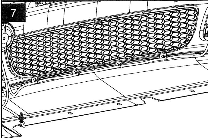
Remove 4 wire harness clips from bottom of lower grille
