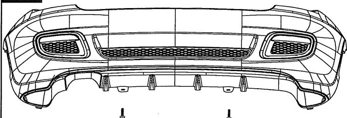
Remove 2 bolts using a T30 Torx bit. Save bolts for re-installation.
