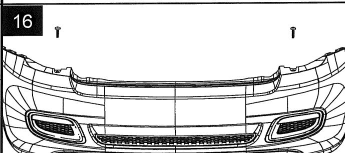
Remove bolts at top of fascia using a T30 Torx bit. Completely remove rear fascia from vehicle. Save bolts for re-installation.
