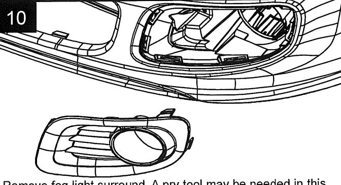
Remove fog light surround. A pry tool may be needed in this step. Install supplied fog light surround (Item C). Ensure all clips are fully engaged by applying pressure at each clip location. Repeat for opposite side.
