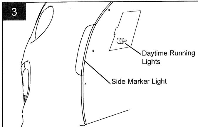
Disconnect headlight wire harness. Disconnect side marker light wire harness. Disconnect Daytime running light wire harness. Repeat for opposite side.
