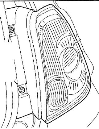
Remove 2 bolts using a 10mm socket. Save bolts for re-installation.
