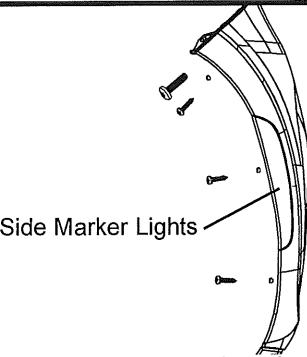
Remove 3 screws from inside wheel well using a philips head screw driver. Remove bolt using T30 Torx bit. Disconnect side marker light wire harness. Repeat for both sides. Save fasteners for re-installation.
