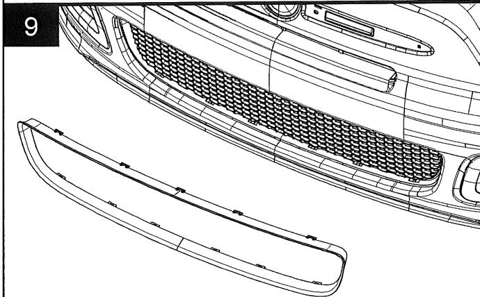
Install lower grille surround (Item B). Ensure all clips are fully engaged by applying pressure at each clip location.
