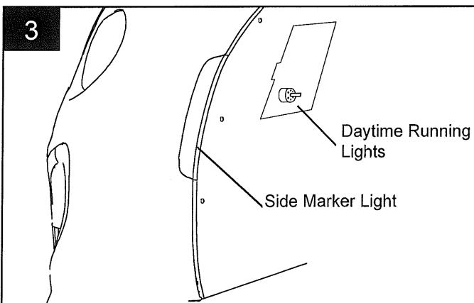
Disconnect Daytime running light wire harness. Disconnect side marker light wire harness. Repeat for opposite side.
