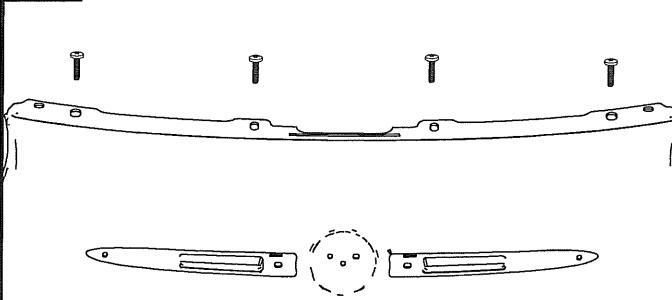
Remove bolts at top of fascia using a T30 Torx bit.
