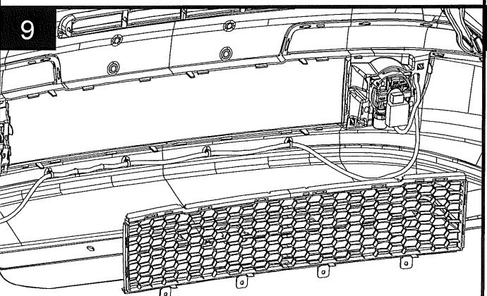
Install supplied lower grille (Item A) to facia. Ensure all clips are fully engaged by applying pressure at each clip location.
