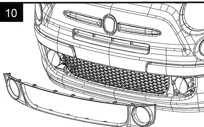
Install supplied grille surround (Item B). Ensure all clips are fully engaged by applying pressure at each clip location.
