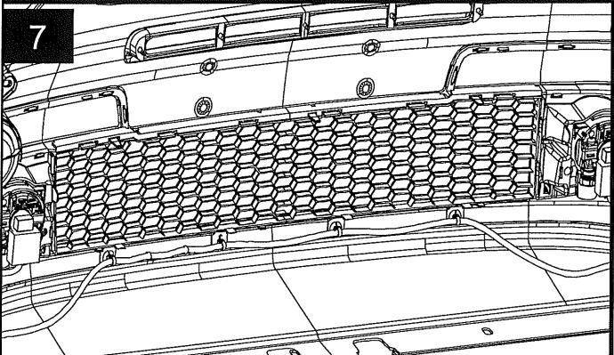
Remove 4 wire harness clips from bottom of lower grille.
