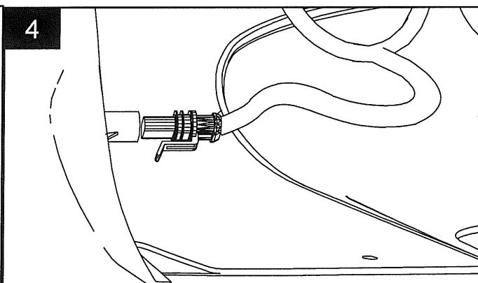
Disconnect fog light wire harness at drivers side of radiator support.
