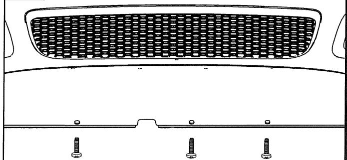
Remove 3 bolts from underside of front Fascia using T30 Torx bit. Save bolts for re-installation.
