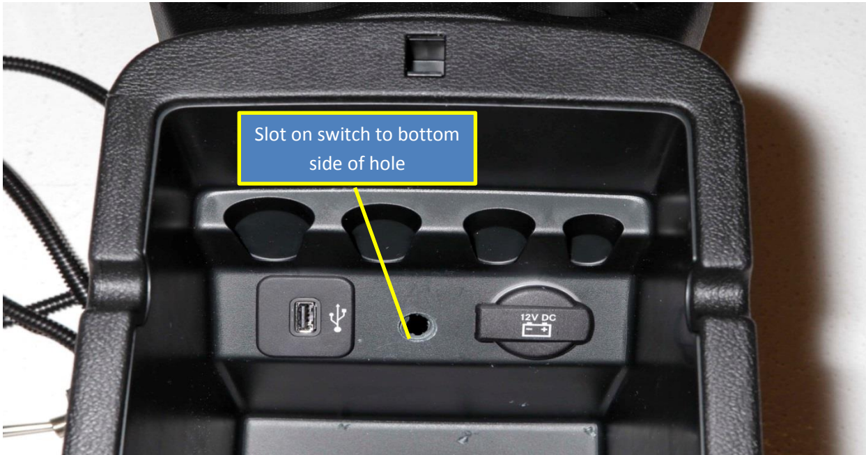
16. Mount switch and switch cover into the center console.
