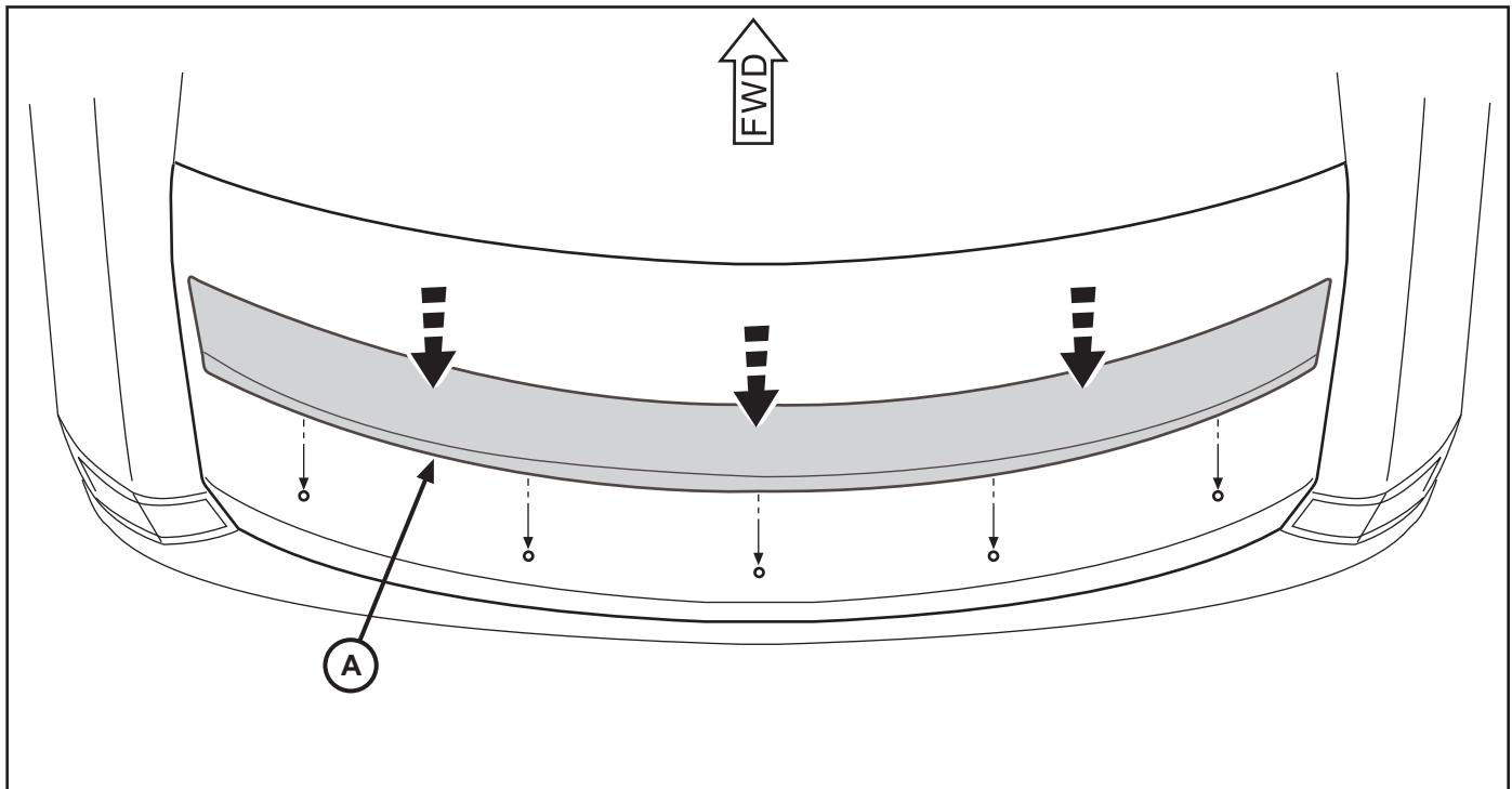
8. Open trunk lid and attach (3) 10mm mounting nuts to spoiler from the inside. Tighten to 6 Nm (4.5 ft. lbs.)
