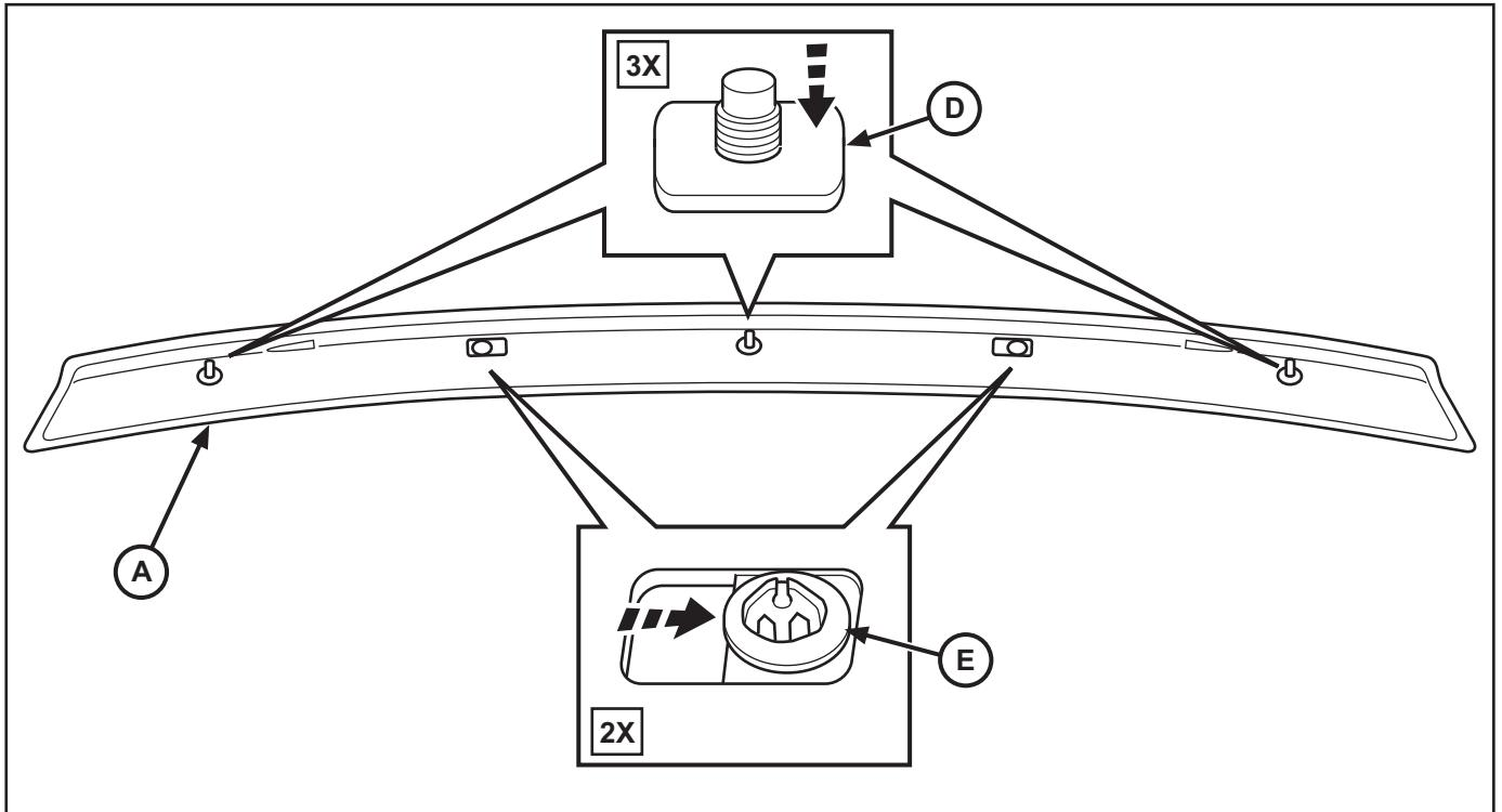
6. Clean spoiler surface with alcohol and allow to dry. Peel away the adhesive liner on one side of an Adhesive Tape pad (F). Place the Adhesive Tape pad on the outside corner of spoiler as shown. Repeat process for the next Adhesive Tape Pad, but position the second pad an equal distance inward from the threaded stud as shown.
