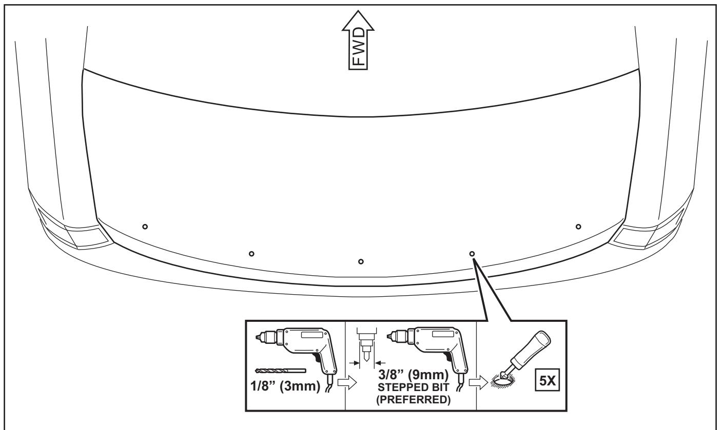
4. Use alcohol to clean the area where the spoiler will be installed. Treat all drilled sheet metal with rust inhibitor outside and inside trunk lid.
