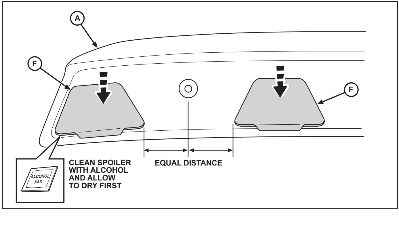
7. Peel the outer adhesive liners from the four (4) Adhesive Tape Pads. Align the Spoiler (A) with the mounting holes and carefully press into place on the trunk lid. Snap the two (2) mounting clips into place.
