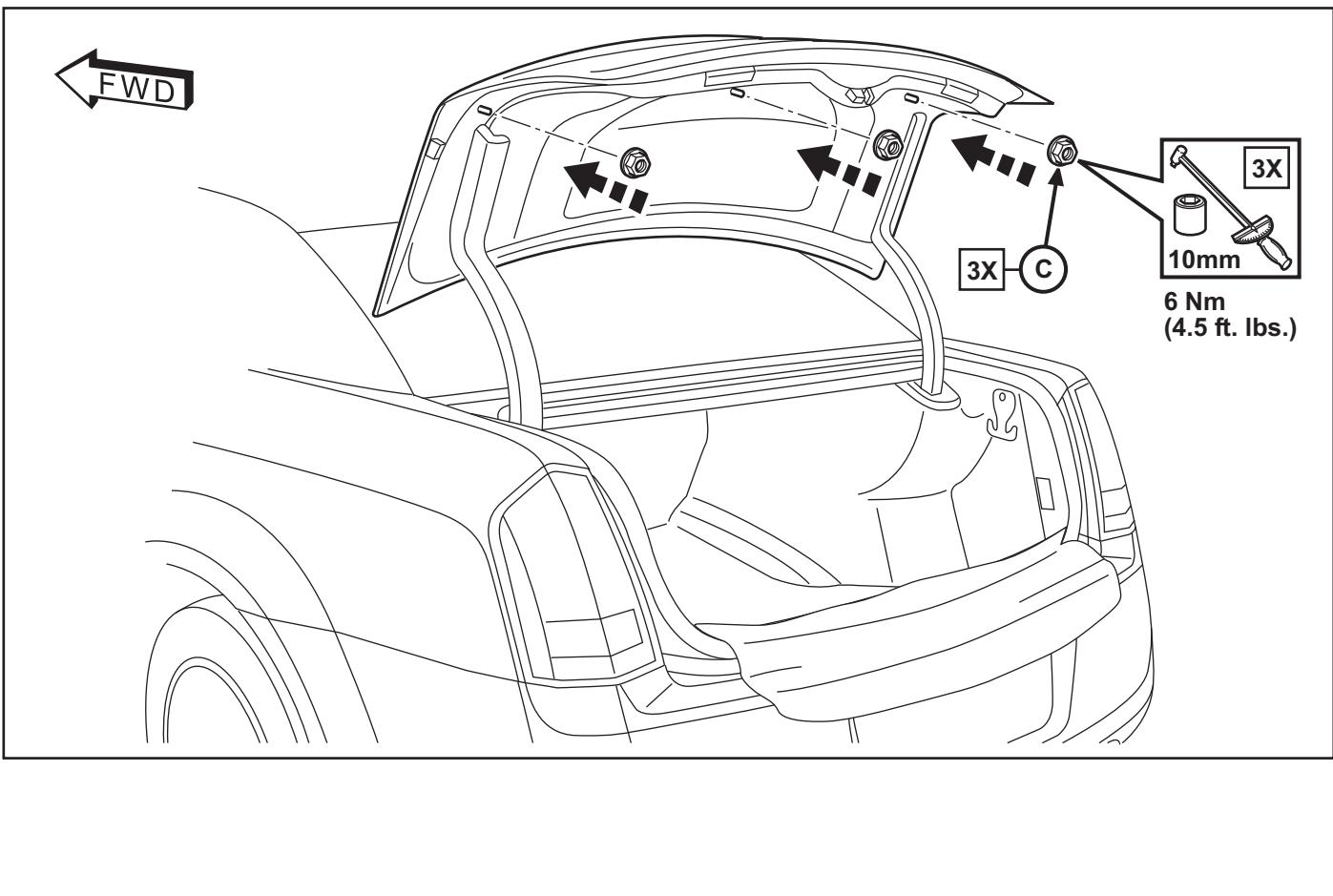
9. Reinstall the insulator panel inside the trunk lid with the (7) push fasteners removed earlier. Reinstall the two (2) bumper pads. Remove drop cloth.
