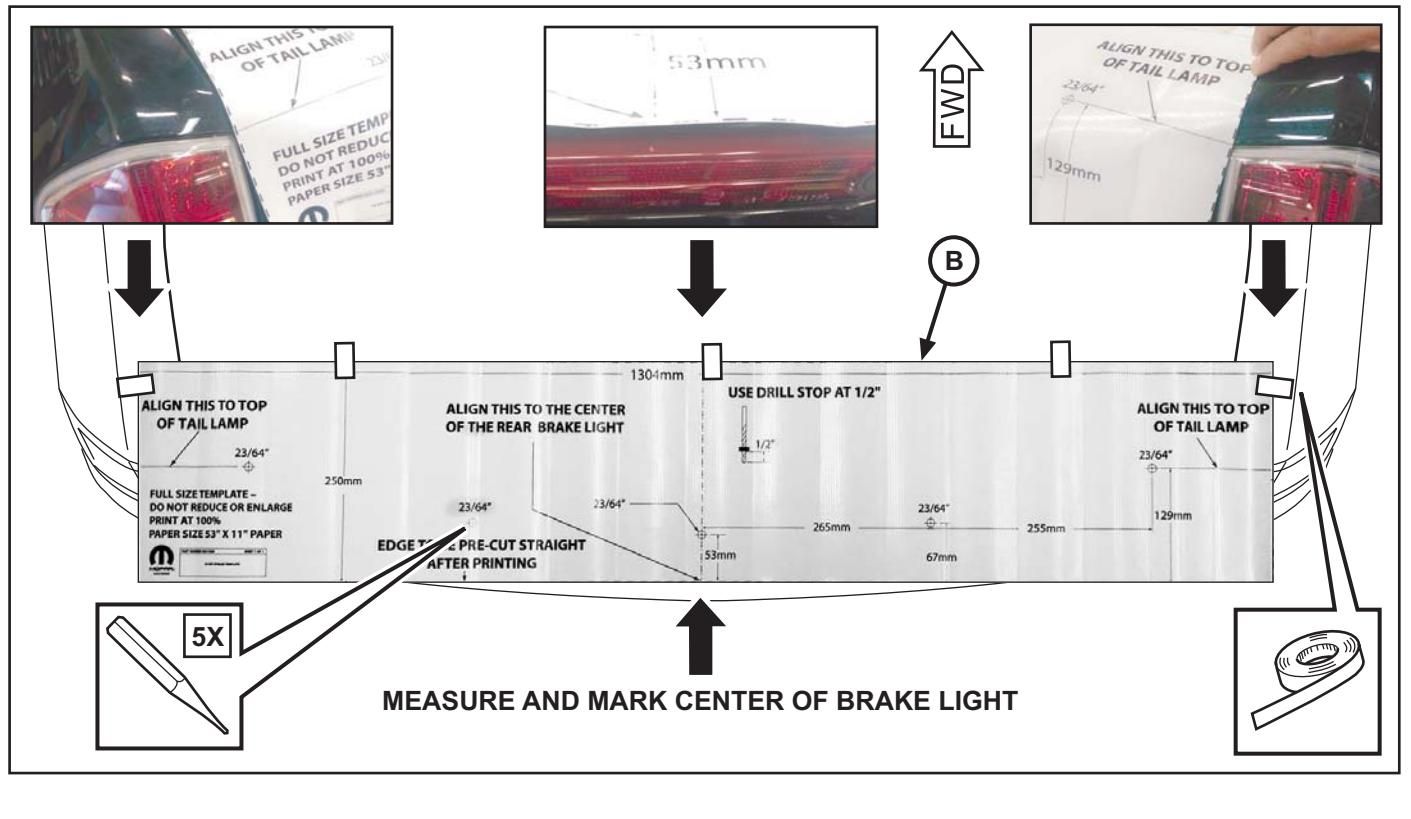
3. Remove the template but **do not discard**. Drill a 1/8" (3mm) pilot hole all five (5) locations. After pilot hole drilling, enlarge each hole to 3/8" (9mm). **A stepped drill bit is recommended**. Use a deburring tool to clean each hole (if required).
