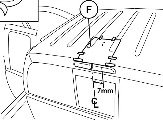
**35** Center template on roof and tape in place
