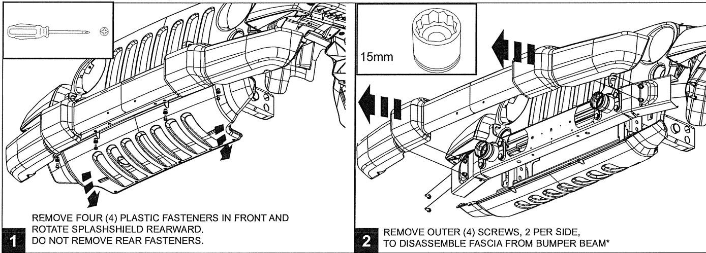
SPLASHSHIELD TO BE MODIFIED FOR INSTALLATION OF TUBULAR FRONT BUMPER
