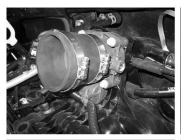
**j)** Attach the reducer coupler to the throttle body and secure with #44 and #48 hose clamps.
