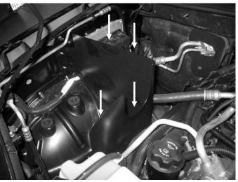
**e)** Insert the heat shield as shown. Align the heat shield to the studs in previous step. The bottom of the heat shield should align with the stud from step 3c.
