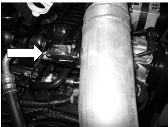
**o)** Install the grommet for the IAT sensor. Reinstall the IAT sensor and reconnect.
