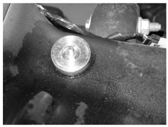
c) Secure the  $\frac{1}{4}$ -20 bolt and washer with the  $\frac{1}{4}$ -20 nut. Tighten.
