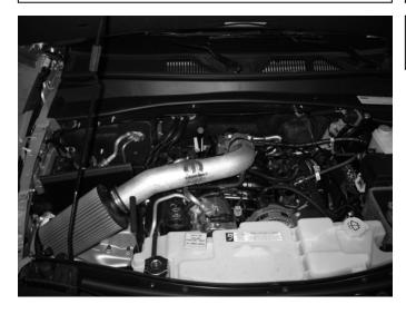
**p)** Attach the filter element and secure with #52 hose clamp.
