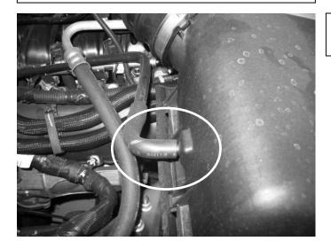
c) Remove the PCV breather tube from the air box. Remove air box and inlet tube.
