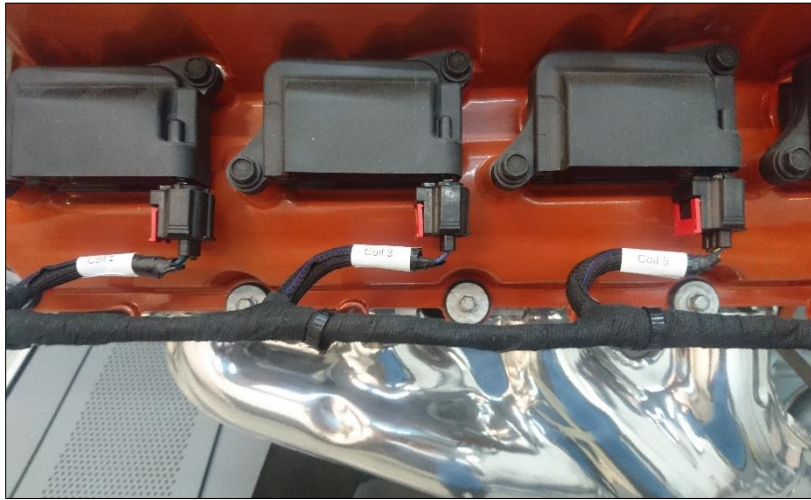
Front Engine Harness Layout for Ignition and Fuel Injection
