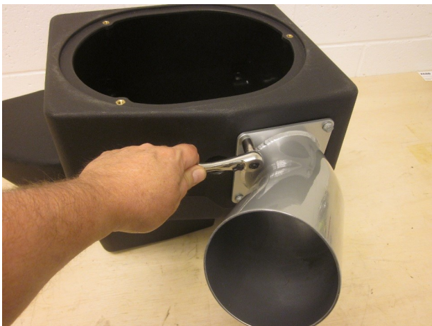
c) Attach the flanged air filter adaptor tube to the MOPAR Air Box as shown with the four (4) M6 bolts provided with Loctite and tighten to 3.5Nm (31 in/lb). Pay attention to the adaptor orientation with reference to the air duct.
