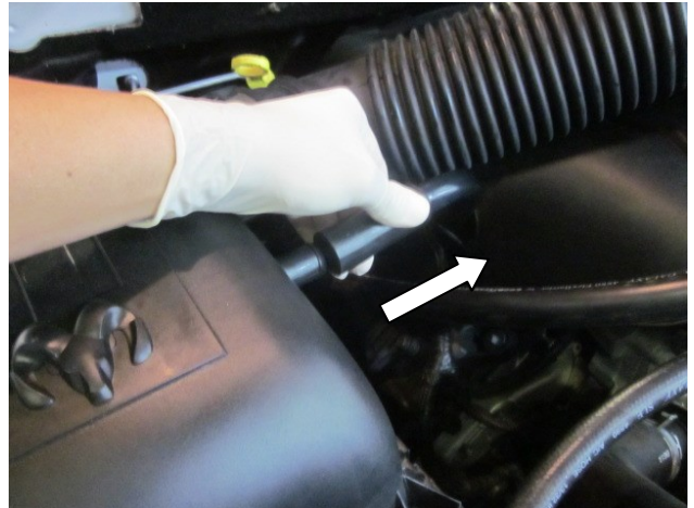
d) Disconnect engine crank case vent hose at the air box.
