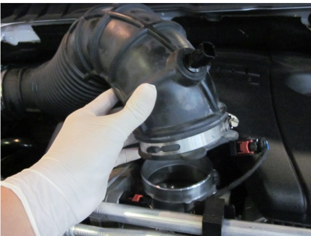
e) Detach the factory air intake hose from the throttle body.
