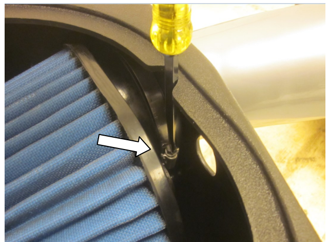
d) Install the air filter on to the air filter adaptor tube inside the air box. Make sure the bead on the adaptor tube engages the groove inside the filter. Do not fully tighten the hose clamp at this point.
