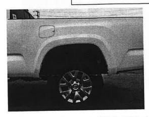
STEP 12: Clean the vehicle body areas with a mild soap and water solution, where the Fender Flares will make contact. Ensure fenders are dry prior to install.
