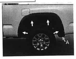
STEP 13: Hold Fender Flare on vehicle in the position of best fit. For models with factory installed Fender Flares, note where above marked holes in Fender Flare align with existing screws in the vehicle. Make special note of "A". Remove the Fender Flare and remove the (4) above indicated screws from the factory flare with a 10mm socket. DO NOT remove the factory flare, the Fender Flare installs directly over the factory flare.
