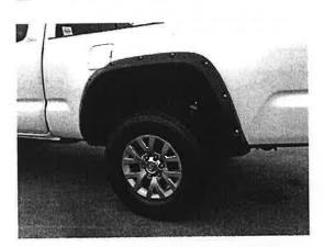
STEP 18: If necessary, make minor adjustments to the flares position to achieve the best fit for your vehicle and to ensure that the rubber seal is sitting flat against the painted vehicle surface. When satisfied fully tighten all screw locations, in the above order in which they were just installed. Repeat install for opposite side.
