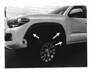
STEP 9: Ensure that the rubber seal is sitting flat against the painted vehicle surface, pay special attention to front area circled above. Using (3) previously removed 10mm screws from STEP 4 or 5, reinstall at above marked hole positions. Do not fully tighten screws at this stage.
