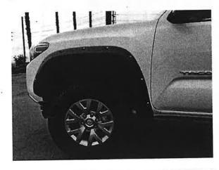
STEP 11: If necessary, make minor adjustments to the flares position to achieve the best fit for your vehicle and to ensure that the rubber seal is sitting flat against the painted vehicle surface. When satisfied fully tighten all (5) screw locations, in the above order in which they were just installed. Repeat install for opposite side.
