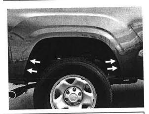
STEP 14: For models without factory installed Fender Flares, remove only the first (4) above indicated screws, from top to bottom of the fender, (2) each side, with a 10mm socket and retain for later re-installation.
