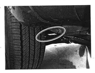
STEP 7: Remove Hooked end Long Clip from hardware kit and install in above shown orientation using the 10mm screw removed from the body sheet metal join in STEP 6 as Special Note area "A". Fully tighten screw and ensure that finished position of clip is horizontal to ground, with the hook end pointing down.
