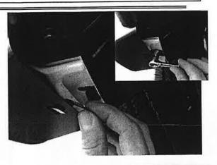
STEP 17: Remove remaining Hooked end Short Clip from hardware kit. Remove 10mm screw from previously noted area "A" in STEP 13 that aligns with mounting slot in Fender Flare. Install hook end of short clip into Fender Flare as shown above and re-install 10mm screw.
