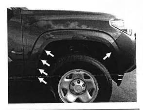
**STEP 5:** For models <u>without</u> factory installed Fender Flares, remove the (5) above indicated screws from the wheel liner with a 10mm socket and retain for later reinstallation.
