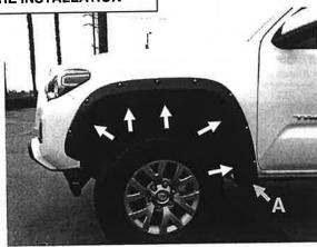
STEP 4: Hold Fender Flare on the vehicle in the position of best fit. For models <u>with</u> factory installed Fender Flares, note where above marked holes in Fender Flare align with existing screws in the vehicle. Make special note of "A". Remove the Fender Flare and remove the (5) above indicated screws from the factory flare with a 10mm socket. <u>DO NOT</u> remove the factory flare, the Fender Flare installs directly over the factory flare.
