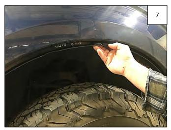
Line up center hole in the Inner Bracket with clip installed in Step 5. NOTE: Driver's side Inner Bracket is marked with an "LF" and the passenger's side Inner Bracket is marked with an "RF".
