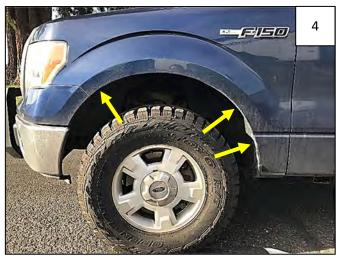
Using a 7/32" socket, remove 3 factory bolts from wheel well. Retain all bolts for reinstallation. NOTE: If you have aftermarket mudflaps, these will need to be removed (and screws retained) prior to flare installation.
