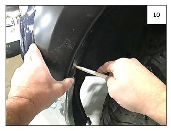
Position flare on fender and use a grease pencil to mark the forwardmost hole location.
