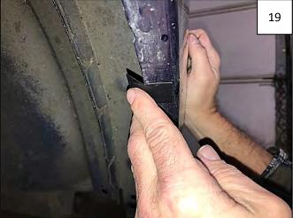
Peel backing from supplied Foam Tab. Center a Foam Tab over each mark made in Step 17.
