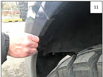
Peel backing from Supplied Foam Tab. Center Foam Tab over mark made in Step 10.
