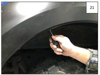
Reposition flare on fender and start 4 supplied Truss Head Screws through holes and into clips.
