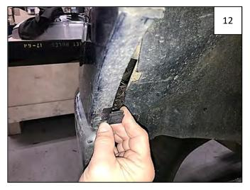
Slide a supplied "S" Spring Clip over foam tab.
