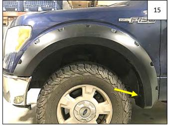
Install a factory bolt through rearmost hole in flare and into factory hole. Apply pressure to flare towards vehicle body and tighten all fasteners.
