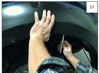
Position flare on fender, holding off vehicle body slightly. Use a grease pencil to mark four holes in flare on fender lip. Holding flare slightly off fender will help with marking the fender lip.
