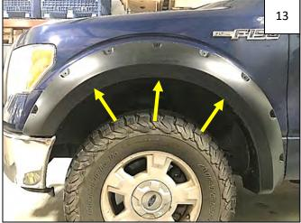
Reposition flare on fender and install three supplied Plastic Retainers through holes indicated by arrows.
