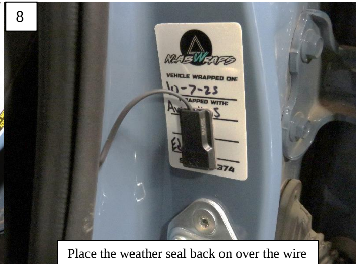
Plug in the connector plugs
