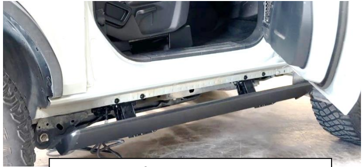
Board is not fully retracted nor deployed
