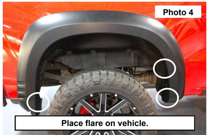
5. Temporarily install the OE screws into (2) of the flare mounting holes to hold into position using the T15 Torx bit.
