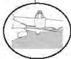
Line up the Center Notch in the Fabric with the Center Notch in the Header
