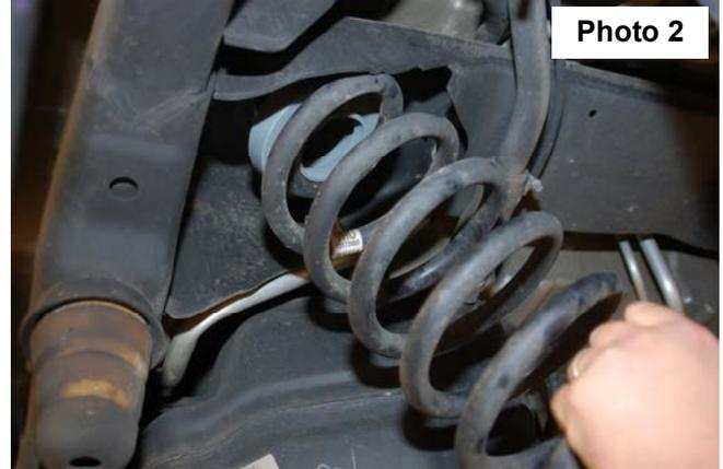
7. Jack up the floor jack to keep the coil springs in position.
