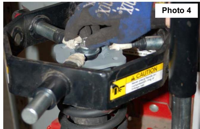
12. Install the supplied 10mm studs in the new Rough Country spacer with the supplied 10mm nuts using a 17mm socket and torque wrench.
