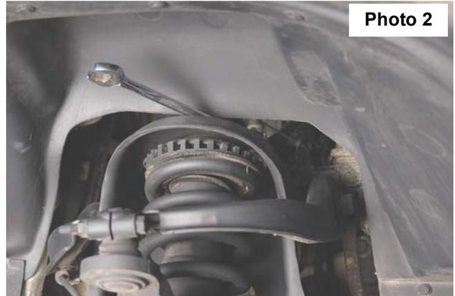
5. Remove the strut from the vehicle.
