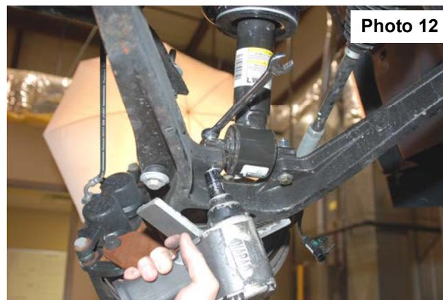
15. Reinstall the sway bar on the lower control arm using a 15mm wrench.
