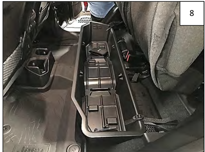
Completed installation of Underseat Storage Box.
