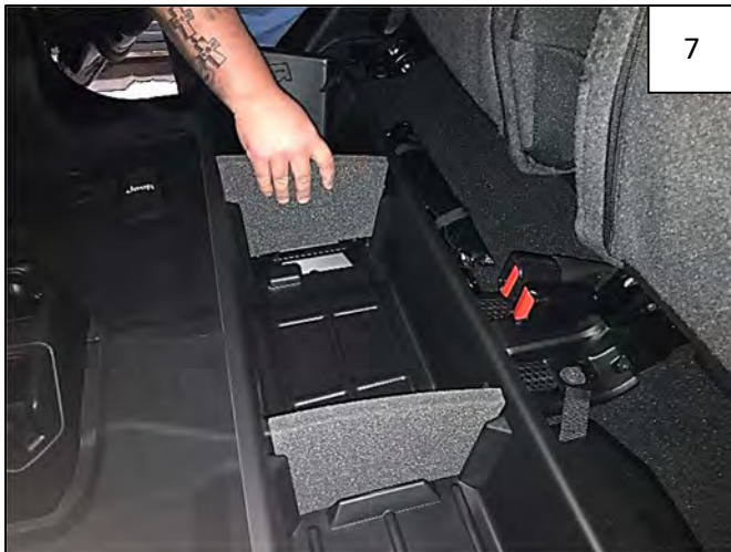
Install Foam Dividers in molded-in slots in Underseat Storage Box.
