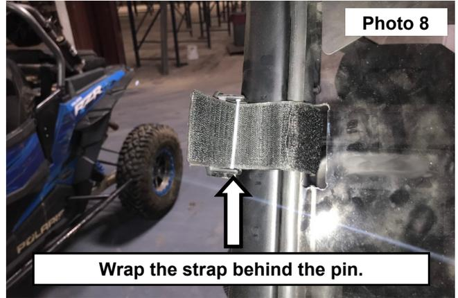
8. Wrap the strap behind the pin in the outer portion of the strap. **See Photo 8.**
