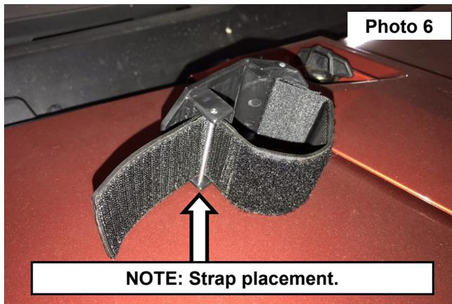
6. **NOTE:** How the strap is wrapped behind the pin. **See Photo 6.**
