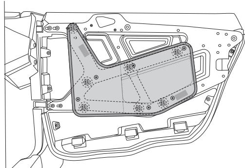
2 Peel off the self-adhesive Velcro hooks and install the bag at the corresponding position on the vehicle, installing the top three screws.
