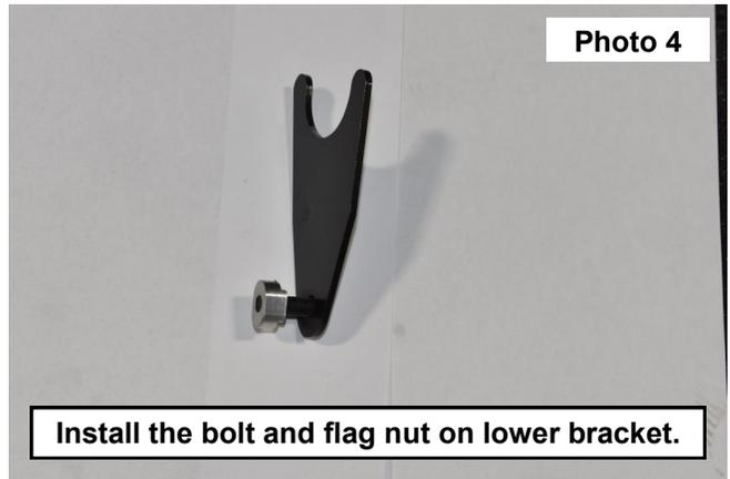
5. Install the bracket over the OE tailgate mount, While installing bracket insert flag nut on bolt into hole and spin until cut outs are flat with the side of hole. Add tension while tighten the bolt with a 5mm Allen wrench. **See Photo 5.**
