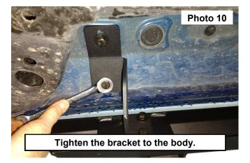
10. Center the step on the vehicle to the desired look. Then tighten using a 13mm socket of wrench. See Photos 11 and 12.
