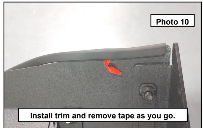
7. Repeat this process for the raised lips down the side rails. You will only put the rubber trim on the edges where the rack will make contact with the roof. The front piece you will stop at the bend line. **DO NOT** install past the bend line. The locations with mounting holes, you will need to leave a 1" gap as shown for bolt head and bracket clearances. **Photo 11 / 12**
